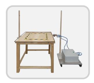
To be used for EMC Tests requiring AC Magnetic Fields Power frequency magnetic fields are generated by AC current flowing in conductors. The normal 50/60Hz mains power cord is a good example, although currents with other frequencies may be present dependant on the application. Magnetic fields, may interfere with equipment operated in close proximity. Typical EUTs are monitors of all kinds.
